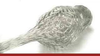
Designed specifically to maintain earth continuity on medium and high voltage jointing systems. The braid is fastened to one end of the exposed armouring. The braids' construction allows it to be pushed back to open and form a cylinder of sufficient diameter to enable the stocking braid to slide over the joint section. Having covered the joint area, the braid is then pulled tight and fastened back over the armouring.
